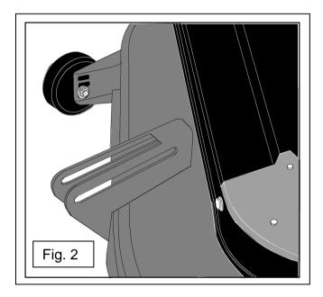
3. Both the front and rear deck-hanging brackets have been changed to accommodate the extra height.
