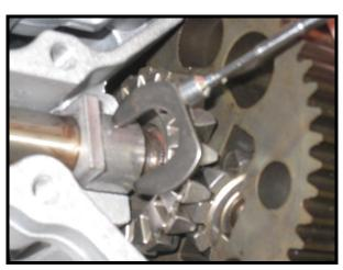
11. Pull axle completely out of transmission housing.
