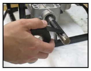
24. Apply a generous coating of grease between the double lips of new seal and over the newly applied tape on axle.
