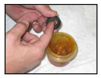
25. Slide seal onto wrapped axle shaft. Seal side with lip retainer spring should be on inboard side.
