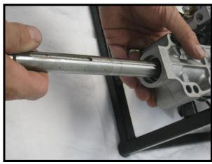
14. Engage axle with differential by aligning splines on end of axle shaft with splines in bore of side gear.
