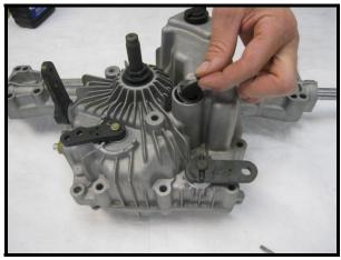
33. Install new plug and seat with a mallet.
