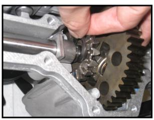
16. Install thrust washer between (inner) axle bushing and diff. side gear.
