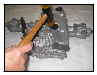
34. Reinstall the fan & pulley stack-up onto the pump (input) shaft. Be sure the components are arranged in the same order as they were removed.
