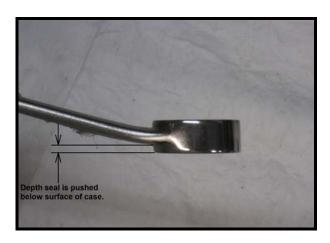
28. Tap against end of wrench to drive seal about 1/8" below surface of housing, to the depth where chamfer on case port ends.
