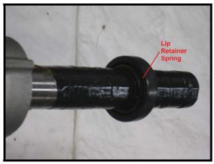
26. After manually pressing seal into case, tap around outer rim of seal with a hammer.
