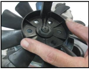
3. Remove black plug by placing the flat blade of a screw driver under its lip and tap upward with a mallet.
