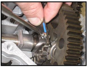
10. Pull outward on axle relieving retainer ring from recess of side gear. Lift ring from axle groove with a magnet.
