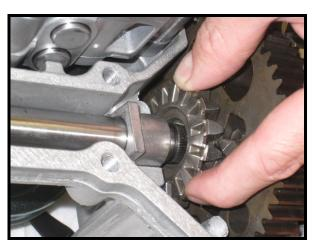
15. Install retainer ring in groove of axle shaft. Then, shift axle so that ring is captured in recess of side gear.
