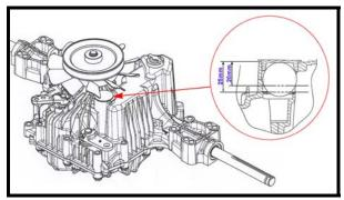
31b. For transmissions with external or remotely located expansion reservoir, oil should be added to the level marked on tank and/or indicated in operators manual.
