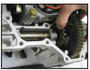
12. Remove (axle) oil seal from transmission case.
