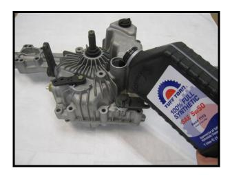
31a. Oil should be added until the level reaches between 20-25 mm (3/4" - 1") from lip of port.
