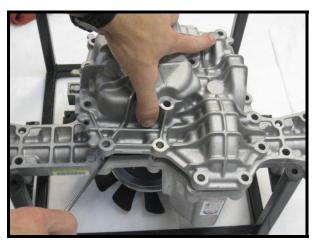
8. Axle shaft must be detached from differential in order to remove it.
