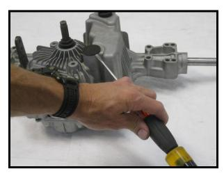
4. Drain used oil from access port by inverting the transaxle.
