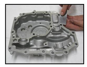
21. Apply a bead of sealant on lower case flange as shown in photo. Be sure to encircle the inner radius of the perimeter bolt holes and completely encircle the (2) interior bolt holes.
