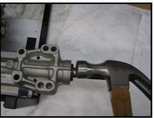
27. Use a box end wrench with outer diameter near same size as seal to drive the seal to its final resting position.
