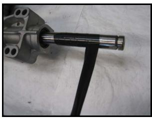
30. Pour new oil into transmission through the access port as shown. Use SAE 5W50 synthetic motor oil included in kit.
