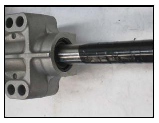
29. Remove tape after seal has been installed.
