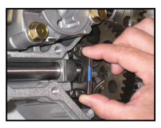
17. Clean metallic particles from the(3) magnets shown.
