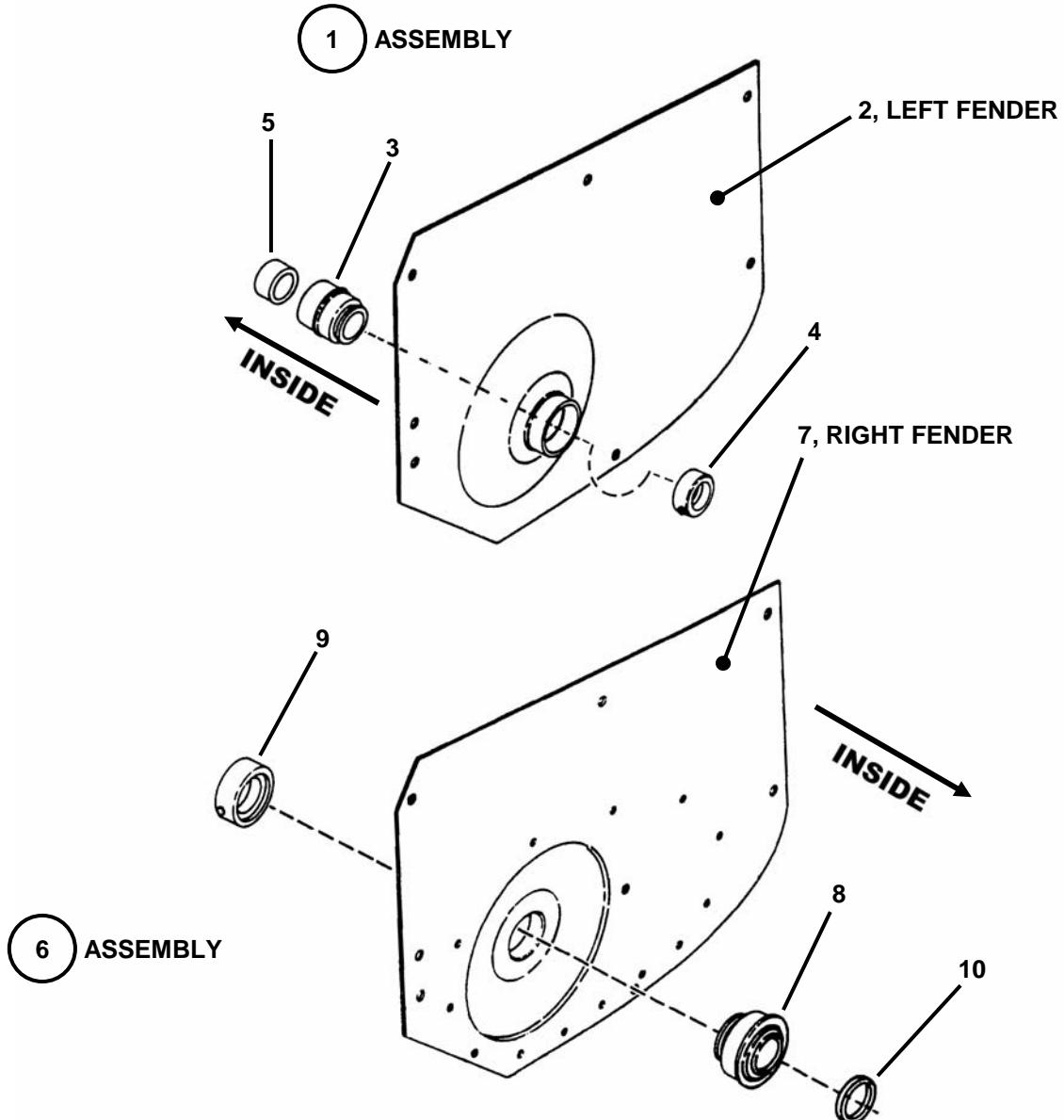
**This kit includes rear fenders with heavy duty ball bearings to replace the standard Riding Mower fenders which have sleeve type axle bushings.**
