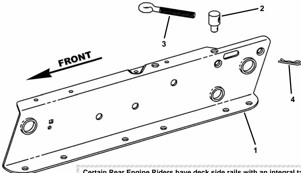
Certain Rear Engine Riders have deck side rails with an integral tab that is used To anchor the blade brake. This specific side rail type is no longer available from part sales. This Deck rail Replacement Kit should be used on all Rear Engine Riders for replacement of the discontinued deck side rail.
