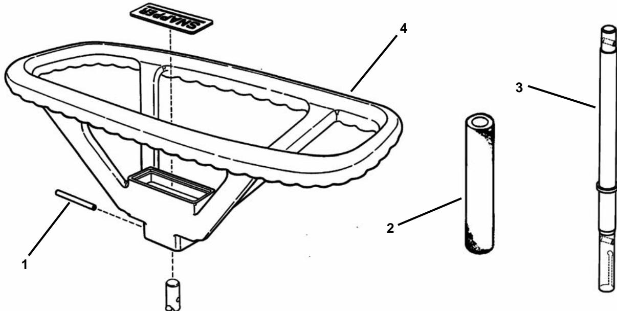
This kit converts Snapper Series 6 and earlier Riders from handle bar type steering to the steering wheel introduced on Series 7 Riders.
