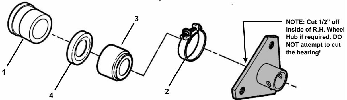
This kit includes an improved axle bearing which is about 1/2" longer in length than bearings used on very early models. This bearing and a shorter wheel hub are furnished on current production.
