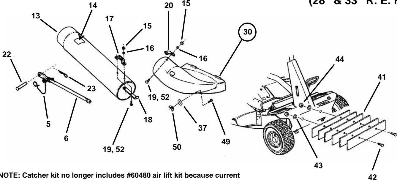
**NOTE:** Catcher kit no longer includes #60480 air lift kit because current Production blades have no air lift bolt holes.
