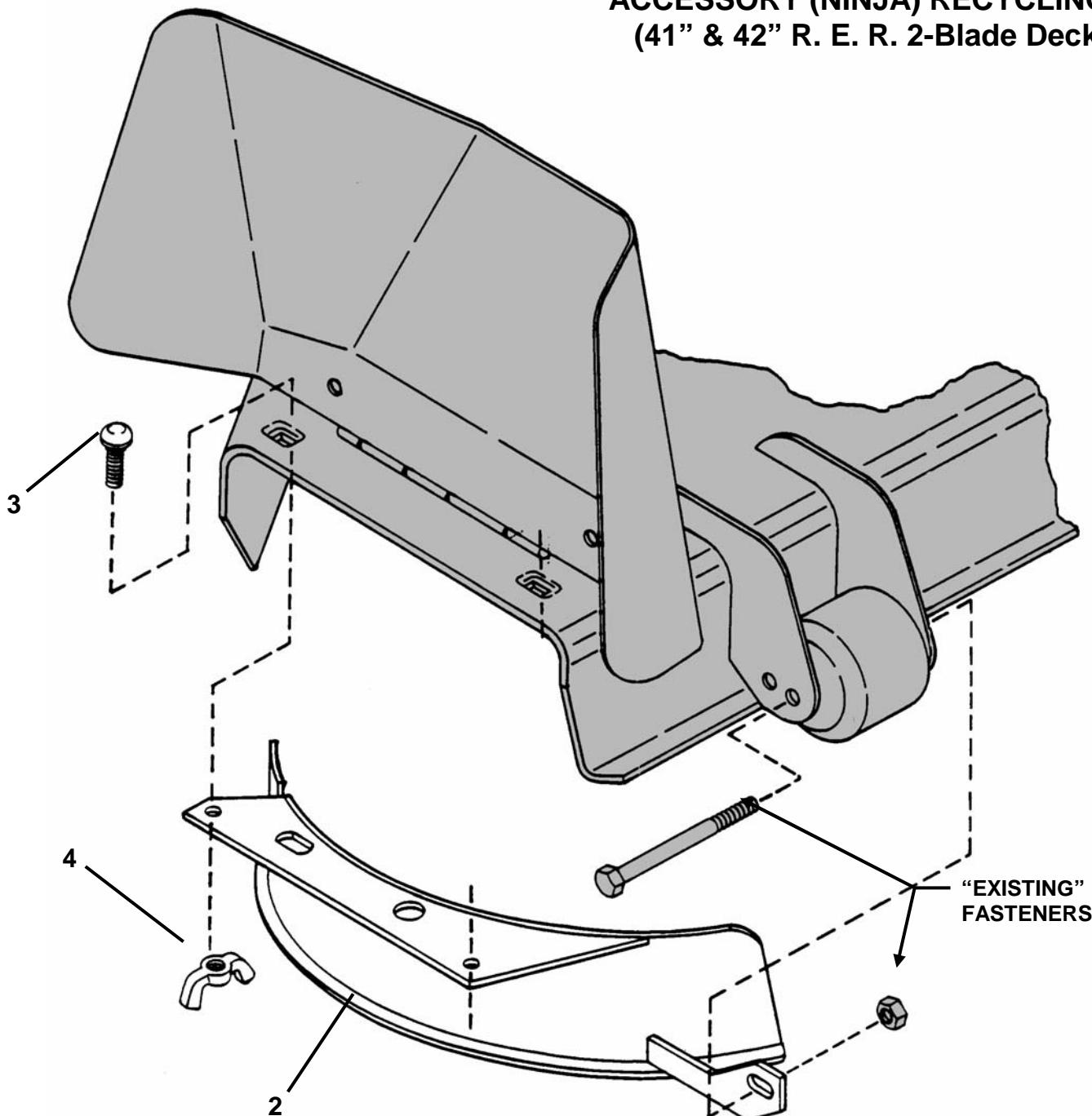
**NOTE:** This kit is intended for use on 41" or 42" 2-blade non-adjustable roller decks.
