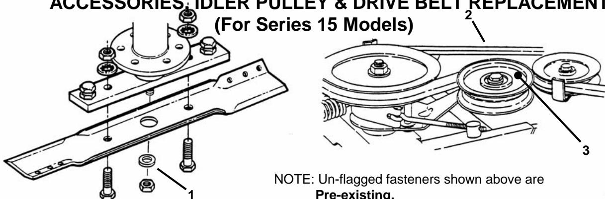
This kit may be used on 26", 28", 30" and 33" single blade mower decks to reduce vibrations on Series 15 Models.
