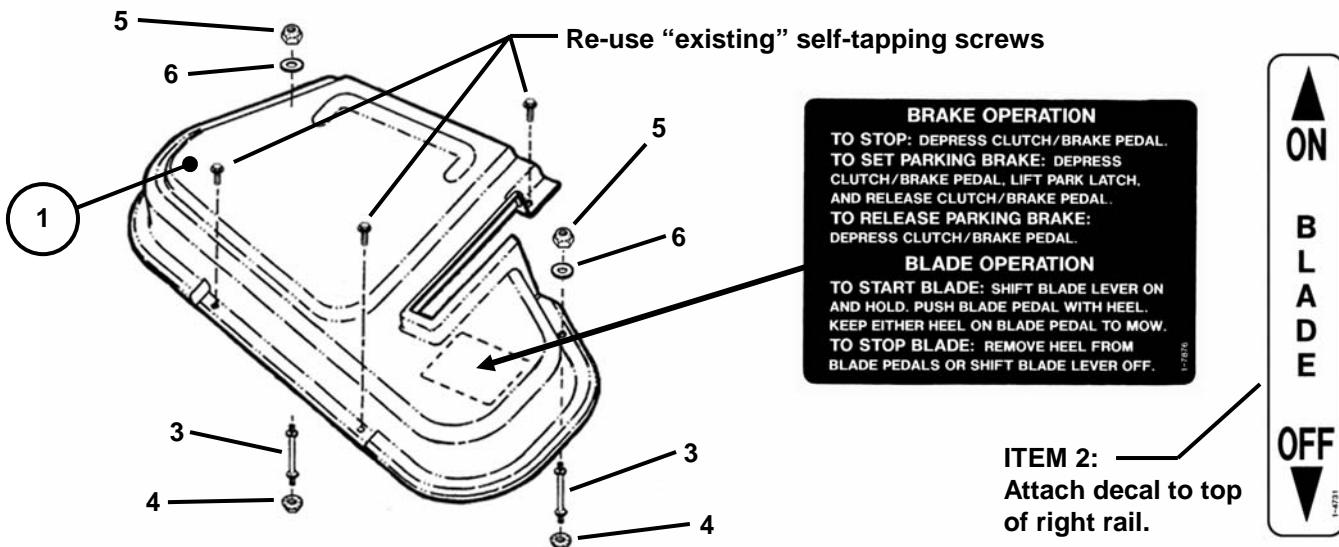
This kit fits all SNAPPER Rear Engine Riders with 41" & 42" cutting decks. This new spindle cover was Designed to allow easy clean up of accumulated debris on top of deck. This cover is more simple to remove to gain access for belt replacement.
