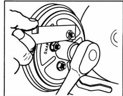
Note: In order to remove or install a smooth clutch friction ring (See Page 80, item 3) it is necessary to prevent the smooth clutch assembly (See page 80, item 1) from rotating while the driven disc retaining nut is being turned. Holding the assembly with vice grip pliers is not recommended as this can cause warpage of the disc and a consequent roaring vibration. Instead, use the smooth clutch tool (3-2392) as shown in the picture at right.
