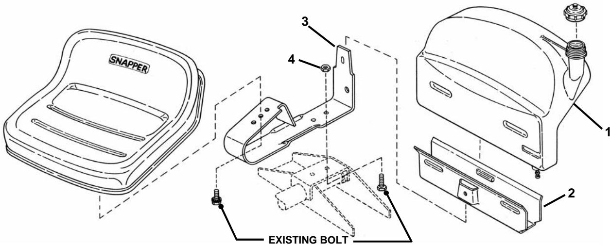
This kit converts the fuel tank on Riding Mowers from side mounting to inboard location behind the operator's seat. Note that the muffler must discharge toward the rear of the rider. This can be accomplished through the use of Muffler Kit 6-0316 on 8HP or 6-0334 on 10-11HP units.
