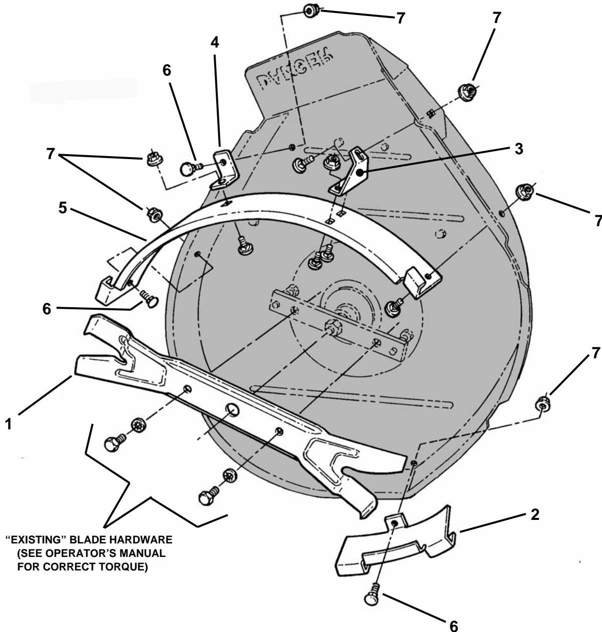
**NOTE: Some 3/8" diameter holes must be drilled to install baffles.
