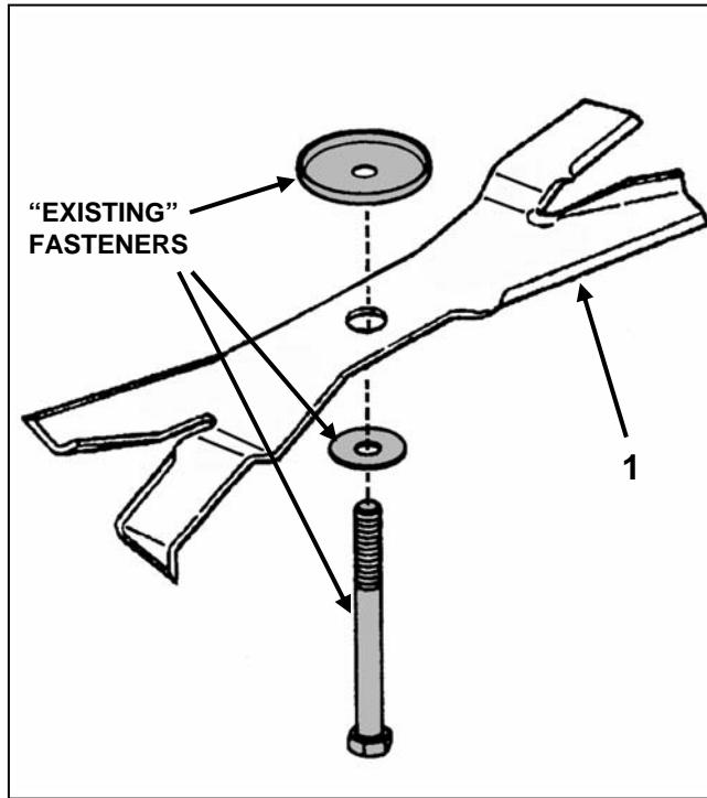
**NOTE: A 11/32" diameter hole must be drilled to install Mulching Cover.
