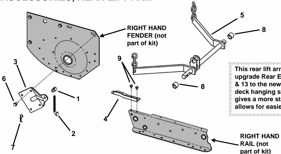
This rear lift arm kit was designed to upgrade Rear Engine Rider Series 12 & 13 to the newer outboard chain deck hanging system. This design gives a more stable deck support and allows for easier adjustments.
